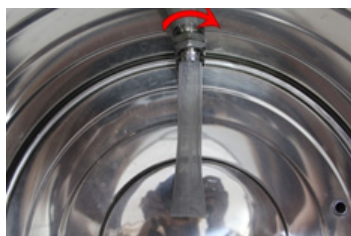
Bazooka mesh filter assembly on tap
