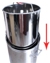
Use the handle to lower the grain basket into the Demacraft. Make sure that the supports on the basket are hooked onto the support ring
