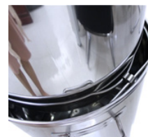
When the mashing is completed, use the handle to lift the grain basket up and hook its bottom
